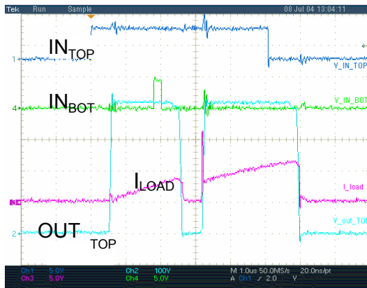
Fig. 12: Switching of one channel pair (TOP1/BOT1) at active hardware interlock
