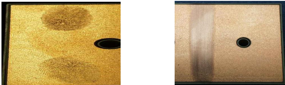
Fig. 7.2 NiAu DCB with fingerprints or discoloration
