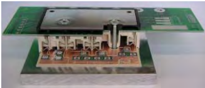
Figure 6: Layout of the ceramic substrate showing chip positions. The internal railing that doubles as a mechanical contact system is shown on the right-hand side.
