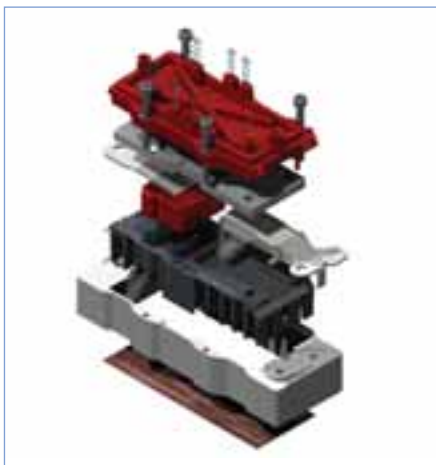
Figure 2. Exploded view of the IGBT halfbridge.
