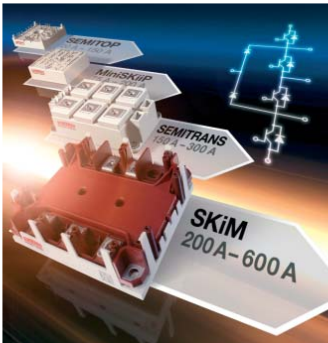
Figure 1: The range includes 600V 3-level modules from 10 kVA to 300 kVA as soldered modules (SEMITOP), spring contact modules (MiniSKiiP) and screw-connection modules with base plate (SEMITRANS) and without base plate (SKiM).
