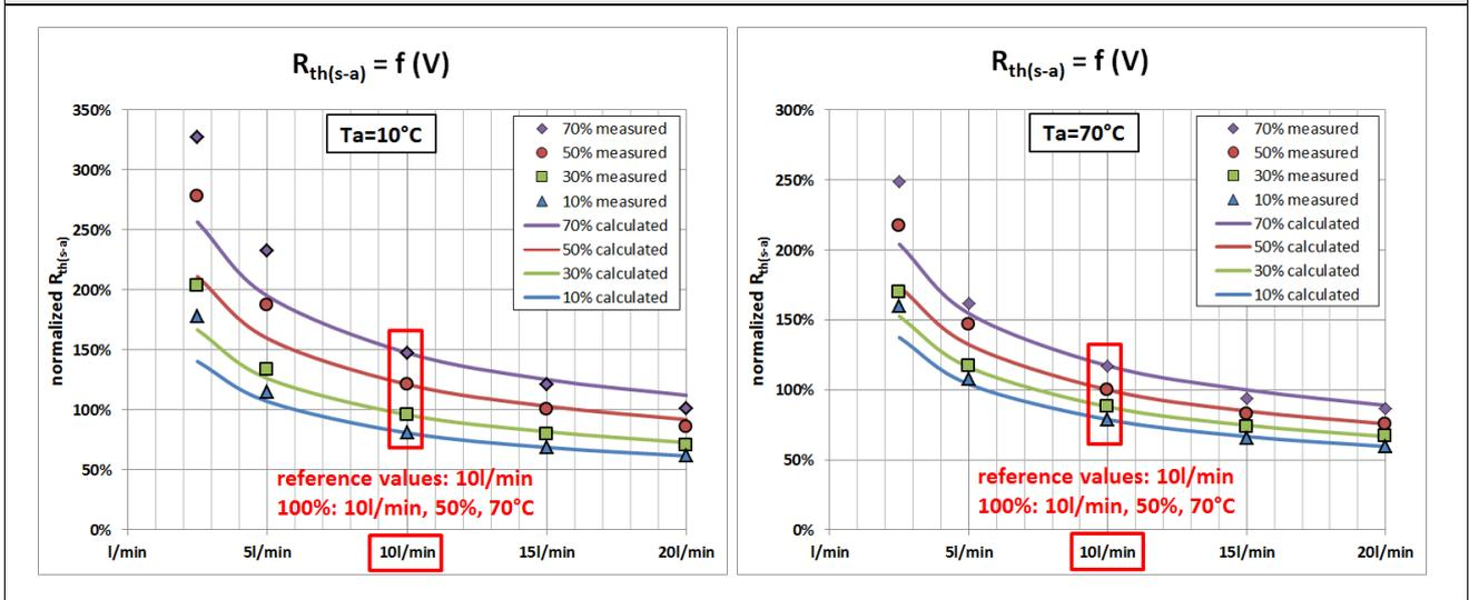
**Figure 7: Normalized  $R_{th(s-a)} = f(V, G, T_a)$ ; measurement vs. calculation (new formula)**
