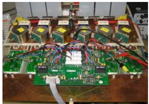
Fig. 17 Test assembly with 6 x SEMiX453GB12E4, individual adapter board, driver and AC terminal in front
