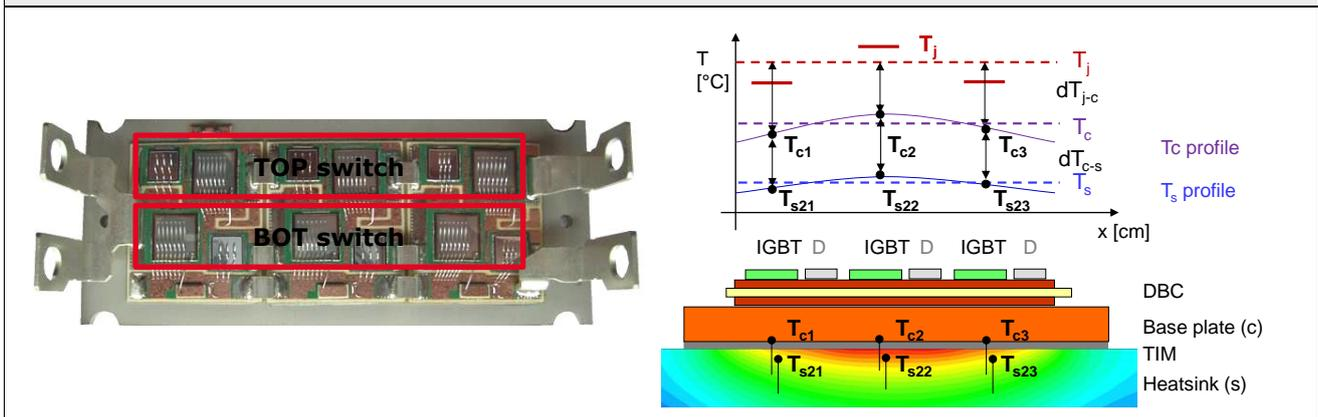
**Figure 4: Measured temperature differences at the three individual TOP switch chip positions and derived  $R_{th(j-c)n}$  and  $R_{th(c-s)n}$  values relative to the average value (100%)**
