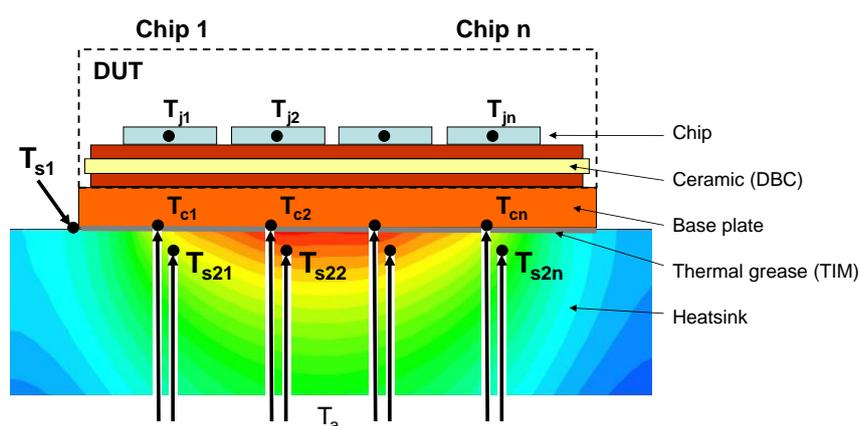
To measure  $T_{cn}$  and  $T_{s2n}$  at the same vertical position underneath the chips different options can be used. The first two have the disadvantage of disassembly and remounting of the module, which is a source for failure where the third has a low failure by a deviation from the chip center position:
