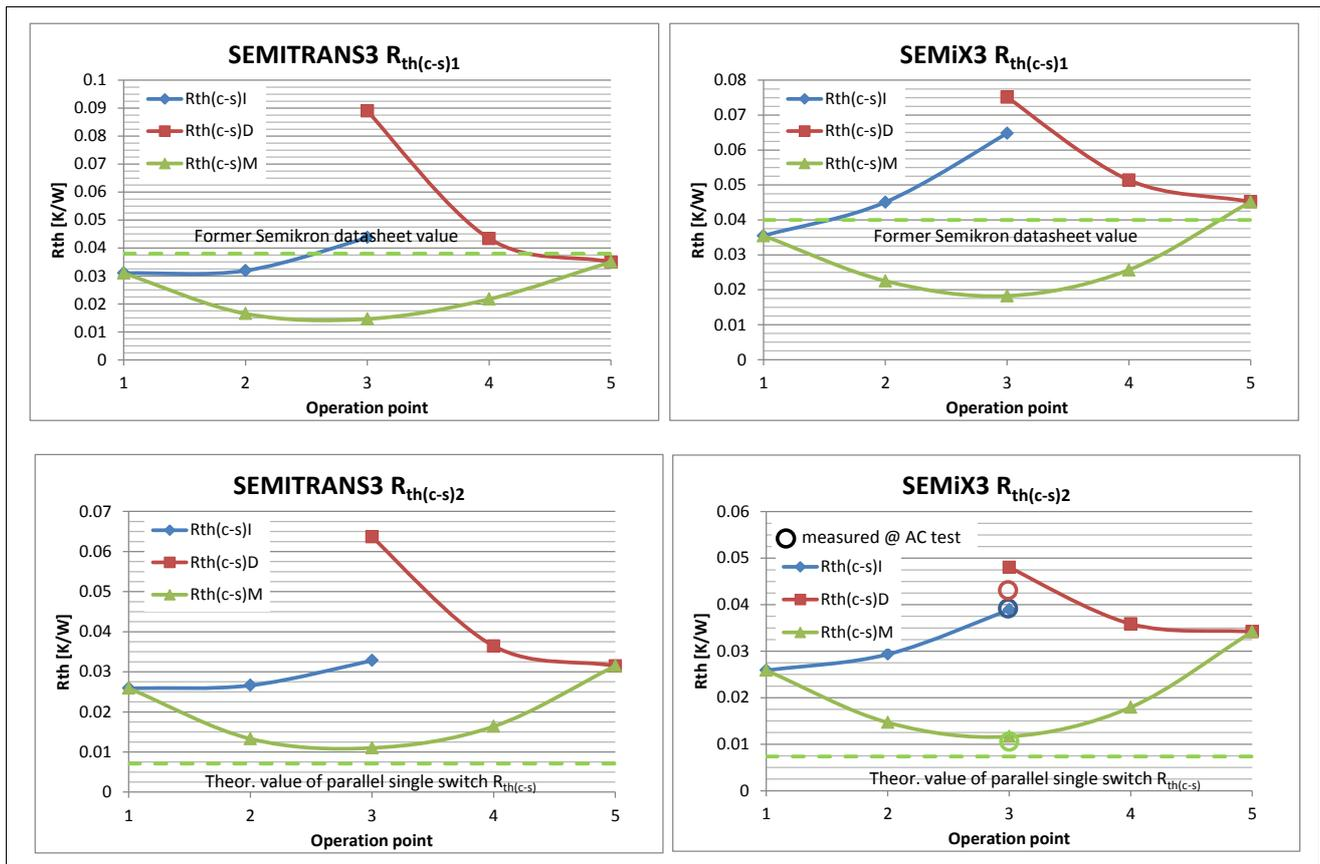
For the different operation conditions following conclusions can be made, taking into account that  $R_{th}$  is inverse proportional to the area  $A$  used for heat transfer ( $R_{th} \sim 1/A$ ):
