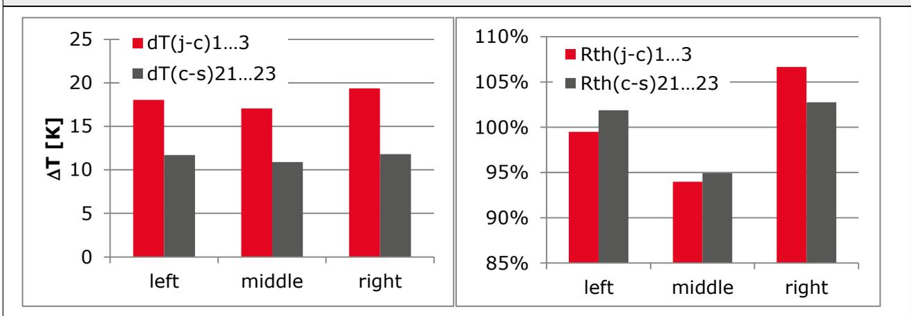
In heatsink rated modules without baseplate are temperature gradients on the heatsink even higher due to the lack of the baseplate's heat spreading effect. Here as well would the position underneath the hottest chip provide the smallest  $R_{th(j-s)}$ . Therefore, the mean values of heatsink temperatures beneath all parallel chips should be used for determination of a switch-related heatsink temperature.
