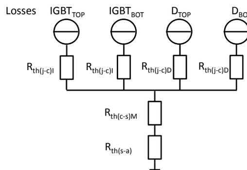
**Figure 11: Thermal equivalent circuit with separate thermal resistance case to heatsink of IGBT- and diode-switch used also for modules without base plate with  $R_{th(j-s)} = R_{th(j-c)X} + R_{th(c-s)X}$**
